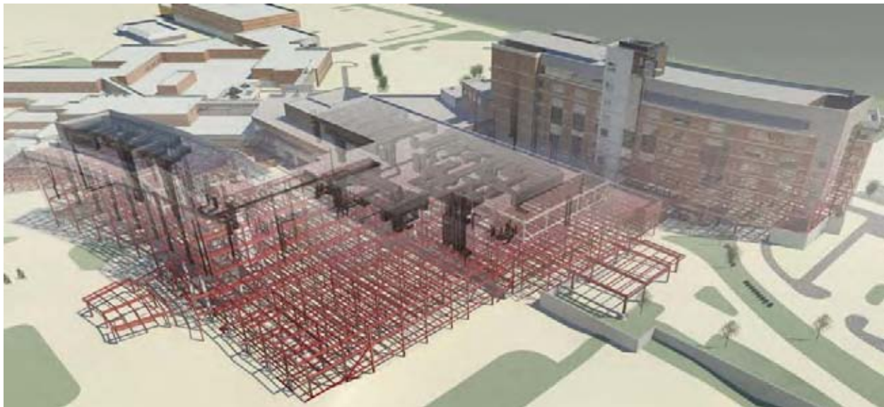
HKS' Revit implementation of the Parkview Regional Medical Center in Indiana. (Courtesy: HKS)
